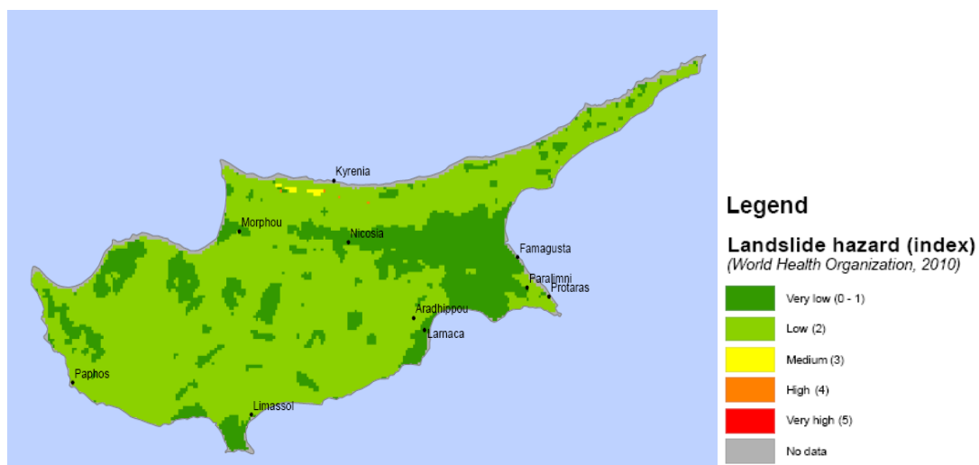
Figure 6.25. Landslide hazard distribution map of Cyprus (WHO, 2010)
