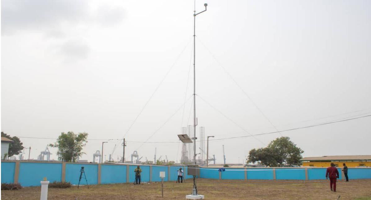
Figure 79: Automatic weather station installed in Accra by GMet under the e-transform project
