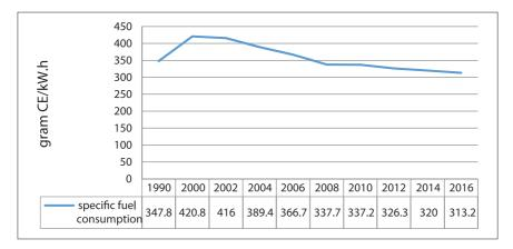
Figure 8.6 Specific fuel consumption for electricity generation of CHPs
