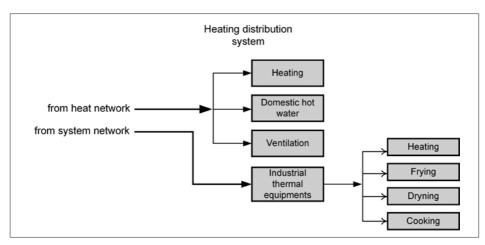
Figure 8.8 Structure of heat distribution system
