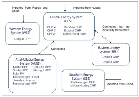
Figure 6.1 Electricity supply system of Mongolia
