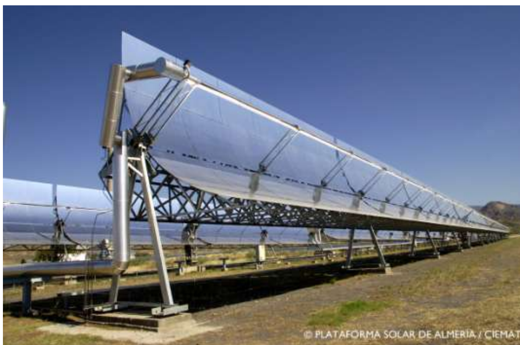
Figure 3. Parabolic Trough collectors installed at Plataforma Solar de Almería (Spain). Photo courtesy of PSA-CIEMAT.
