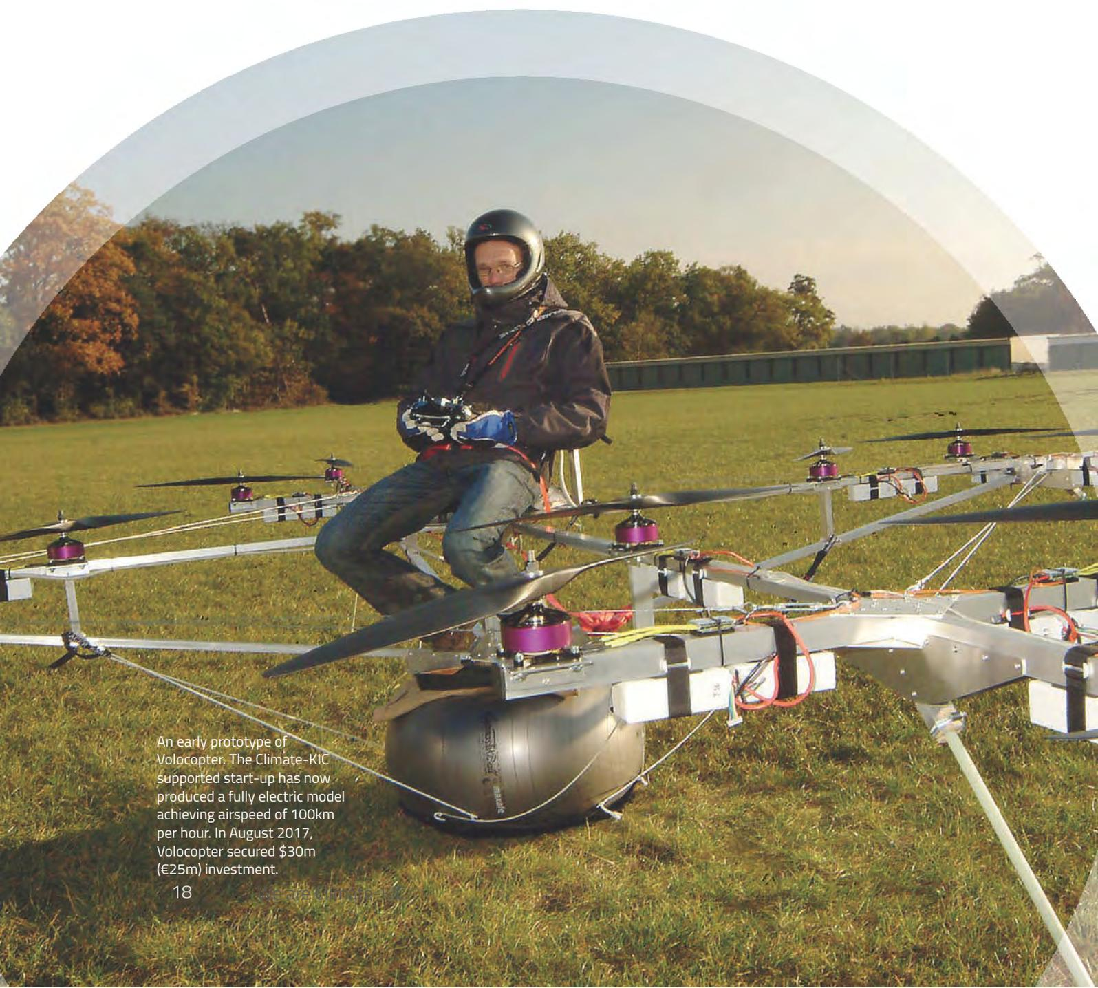
An early prototype of Volocopter. The Climate-KIC supported start-up has now produced a fully electric model achieving airspeed of 100km per hour. In August 2017, Volocopter secured \$30m (€25m) investment.
